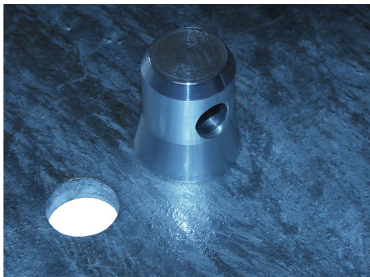
Machined aluminium alignment spigots with retaining bolts matches up with NBS-SAL bolts
