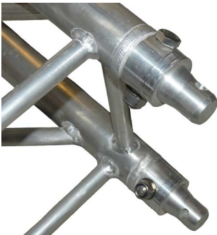
The joining sockets at both ends and and bullets located at one end for ease of installation. Each bullet and joining socket have a nyloc secured bolt for maintaining joint.
