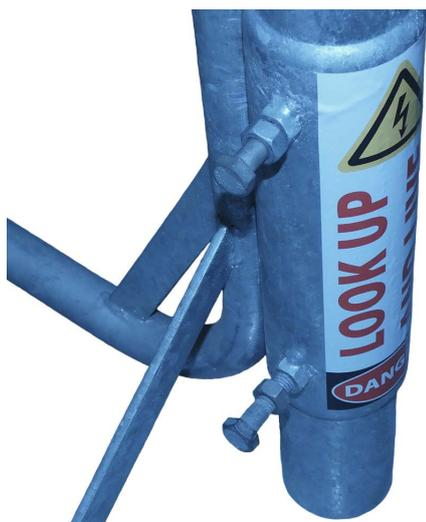
2 x locking bolts supplied in the base to secure your masts once inserted to stop movement. Bolts are to gently squeeze masts against socket tube wall. Do not overtighten as to crush the telescopic tube.
